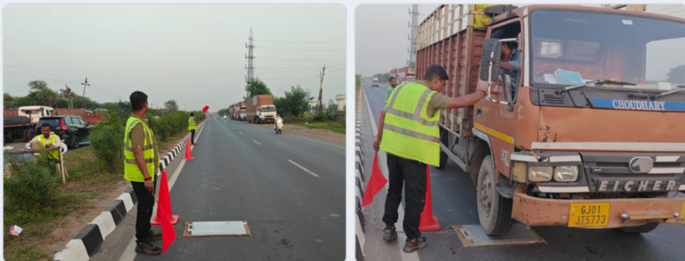
Figure 2.3. (a) and (b) Axle load survey being conducted
